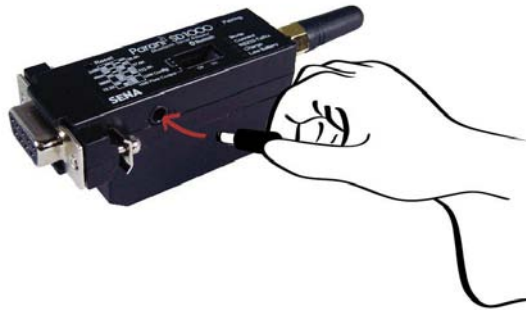
Figure 2-2 Connecting Power to Parani-SD1000
