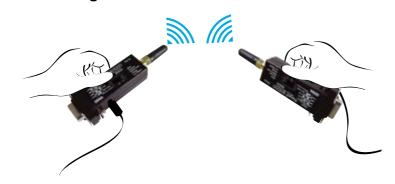
Parani-SD provides Pairing Button for instant configuration without a PC to make an automatic connection between two Parani-SDs. We will refer to the two Parani-SDs as SD1 and SD2, respectively. In pairing status, SD changes IAC value automatically.
